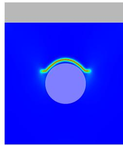
**Phase 2 : Brutal onset.** At  $t \sim 0.28$ , a crack of finite length brutally appears near the top of the inclusion. The crack is symmetric with respect to the 2 axis; it is not straight.
