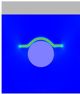
**Phase 3 : Progressive and symmetric evolution of the crack.** When  $t$  varies between 0.28 and 0.38, the crack progressively grows in the matrix. The evolution is smooth: the surface energy increases smoothly, while the bulk energy is nearly constant. The propagation is symmetric but not straight.
