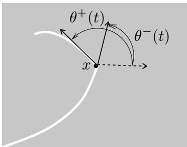
Figure 2: The crack propagates at  $t$  from the tip  $x$  in the direction  $\theta^+(t)$ . If  $\theta^+(t) \neq \theta^-(t)$ , kinking occurs, whereas, if  $\theta^+(t) = \theta^-(t)$ , there is no kinking.
