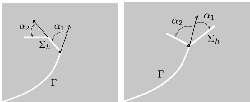
Figure 5: Testing stability with a kinked or a branched add-crack
